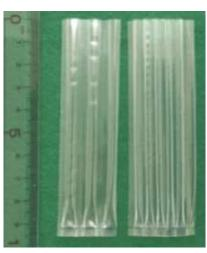
Left: 3-cell type, right: 6-cell type. Cells are filled with solution, loaded with an inner container filled with crystallization sample, and heat-sealed.
