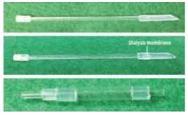
Capillary for the counter diffusion method Capillary for the dialysis method Large-bore capillary for neutron diffraction
